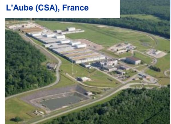
At *Centre de l'Aube* in France, site geology, facility design and waste limits are in place to meet safety requirements.
