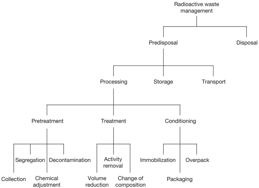
**conditioning.** Those *operations* that produce a *waste package* suitable for handling, *transport, storage* and/or *disposal*. *Conditioning* may include the conversion of the *waste* to a solid *waste form*, enclosure of the *waste* in containers and, if necessary, provision of an *overpack*.
